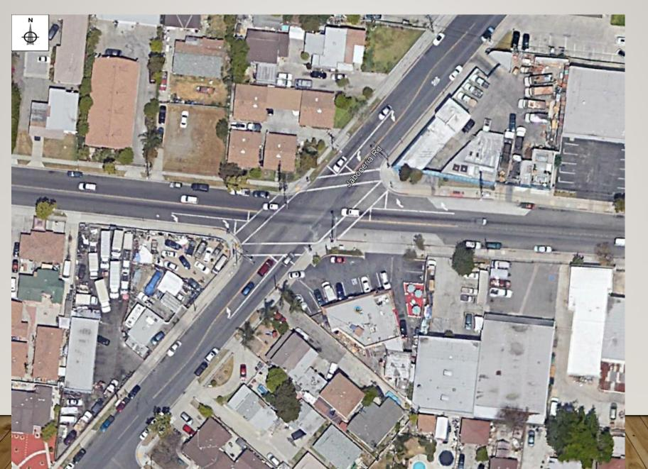
NB/SB Jaboneria has thru/right turn lanes with dedicated left turns EB/WB Clara has thru/right turn lane and dedicated left turn lanes The signal operates as a split phase for Clara
