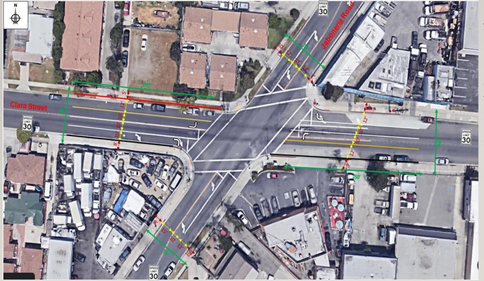
WB/EB Jaboneria to be Restriped to allow Dedicated left/thru/right lanes and change signal operations to normal versus split phase
