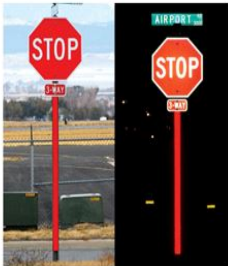
Figure 5 - Reflective Tape for Stop Signposts
